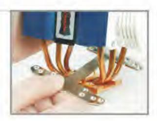
Place the heat sink on the CPU core as shown.
